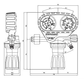
Pressure gauges are precise measuring instruments. They are the most sensitive regulator components exposed fully to the industrial environment. Robust rubber cap gives optimal protection against potentially rough handling. Consumption of the spare pressure gauges is three times lower in the markets where using gauge protections is a common habit already today, compared to markets with not protected regulators. The savings are even more significant if customer changes regulator completely.
