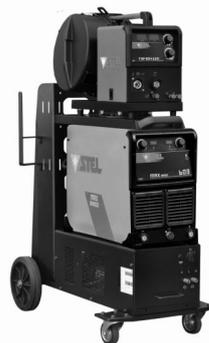
In this mode the generator behaves as a constant voltage generator, to weld in MIG mode it is necessary to connect it via a cable bundle to a compatible wire feeder. In case of connection with a wire feeder it is the power supply to take control of the welding parameters.
