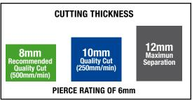
The declared cutting data are equal with internal or external compressor
