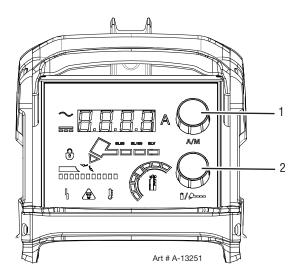
1. Press and release the upper knob without turning to enter the mode selection menu. Place the system in one of the four cutting modes available by pressing and releasing the knob until you reach the desired mode.:
