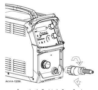
Connecting the Torch to the Power Supply
