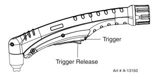
6. Bring the torch within transfer distance to the work. The main arc will transfer to the work, and the pilot arc will shut OFF.
