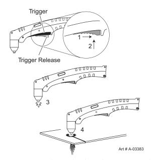
8. Cut as usual. Simply release the trigger assembly to stop cutting.
