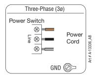
Three Phase Input Power Wiring
