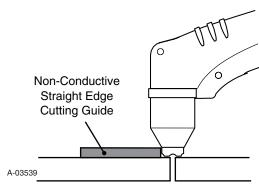
Using Drag Shield Cup With Straight Edge
