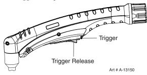
7. Bring the torch within transfer distance to the work. The main arc will transfer to the work, and the pilot arc will shut OFF.
