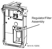
1. Remove power from the power supply; turn OFF the gas supply and bleed down the system.
